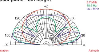
90° Elevation Max. Gain = 3.49 dBi 23° Elevation Max. Gain = 7.72 dBi 16° Elevation Max. Gain = 7.51 dBi
