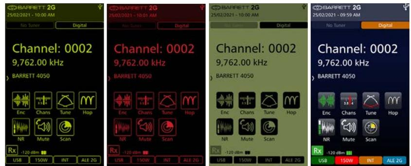
The 4050 HF SDR software has four separate theme modes for use in different ambient light conditions. The screen can also be turned into landscape format via the user interface, if required.
